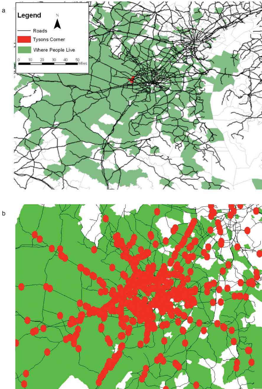
FIGURE 4.9 Using agent-based models to explore rush-hour congestion: (a) road and Census data used for model inputs; (b) zoomed-in section of (a) with agents (red circles) moving towards Tyson's Corner and causing traffic jams
